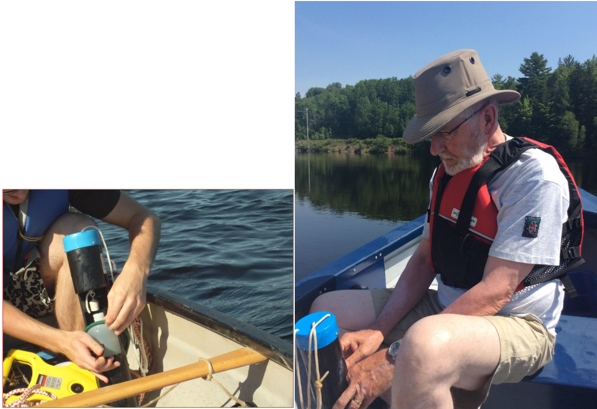
FIGURE 2-2 SAMPLING DEVICE USED TO COLLECT WATER SAMPLES FROM MONITORED LAKES
