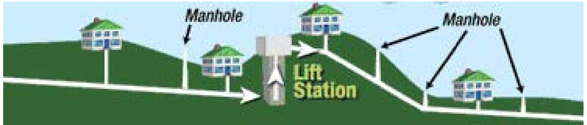
Traditional Gravity Sewer System
