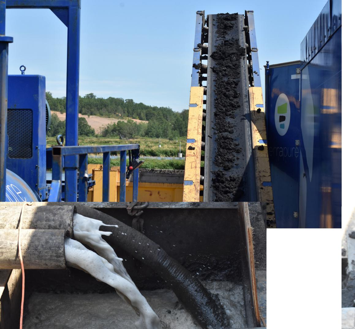
The sludge extracted from the primary sewage lagoon is cycled through a spinning centrifuge for dewatering.
